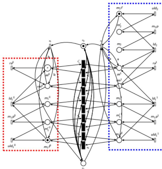
RMS with two machines (based on basic GPSNs).
